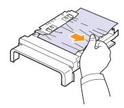
If the paper does not come out with the duplex unit, remove the paper from the bottom of the machine.
